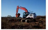
"The 160 X4 delivers up to 5% faster cycle times than its predecessor," said Nori Kumagai, LBX Product Manager. "We redesigned the control spools and incorporated spool stroke control (SSC) functions into the hydraulic system to reduce pressure loss and distribute oil more smoothly. Two electrically-controlled Kawasaki variable-displacement axial-piston pumps and one Kawasaki gear pump assure that hydraulic flow gets delivered
