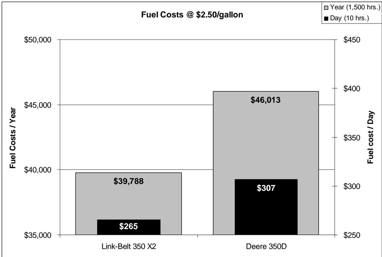
Fuel cost per day was calculated by multiplying the fuel consumption per hour by 10 hours by \$2.50 per gallon of diesel. Fuel cost per year was calculated by multiplying the fuel consumption per hour by 1,500 hours by \$2.50 per gallon of diesel.
