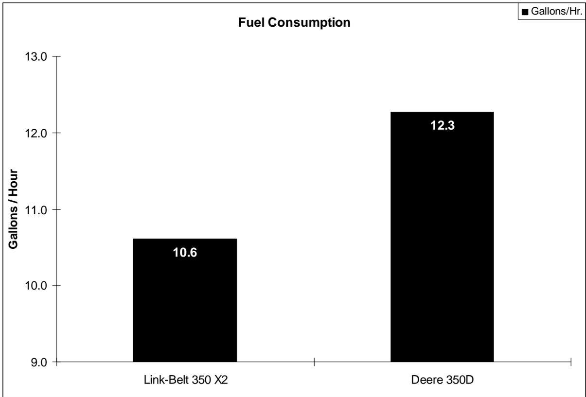
Fuel consumption was measured utilizing a calibrated fuel meter installed on each machine. Machines were operated in the highest work mode setting, running at the highest engine RPM, with 100% utilization.
