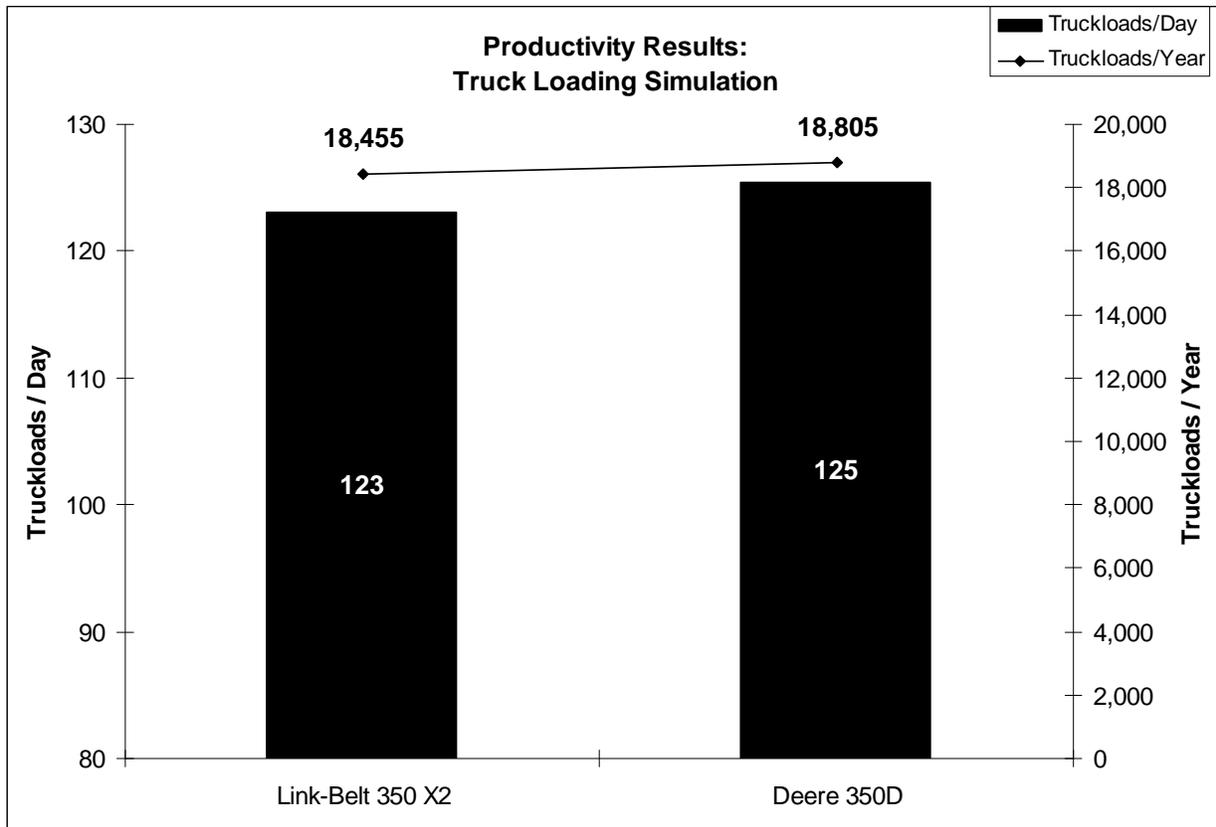
Productivity was based on a fully-loaded 30-ton size truck with a heaped capacity of 21.6 yd<sup>3</sup>. The number of truckloads per day was calculated by multiplying the number of estimated\* cycles per hour by 10 hours per day for each machine by the stated capacity of the bucket installed on each machine. The number of truckloads per year was calculated by multiplying the estimated number of truckloads per hour by 1,500 hours.
