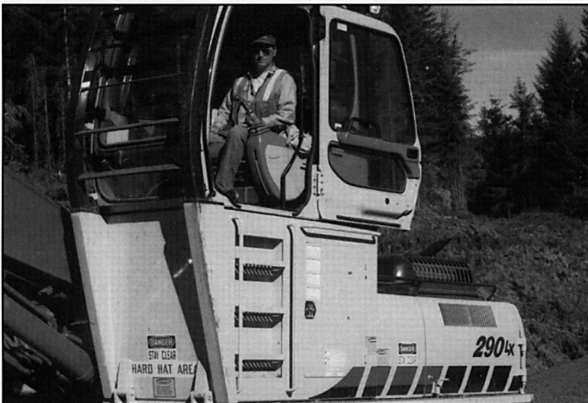
DARIN SCHMELTZER OPERATES THE LINK-BELT 290 LX LOADER ON THE F & B LOGGING GROUND SIDE. HE CITES THE WEIGHT OF THE MACHINE AND THE SWING TORQUE AVAILABLE TO HIM AS IMPORTANT FEATURES ALLOWING EFFICIENT AND EFFECTIVE OPERATION AT THE LANDING.
