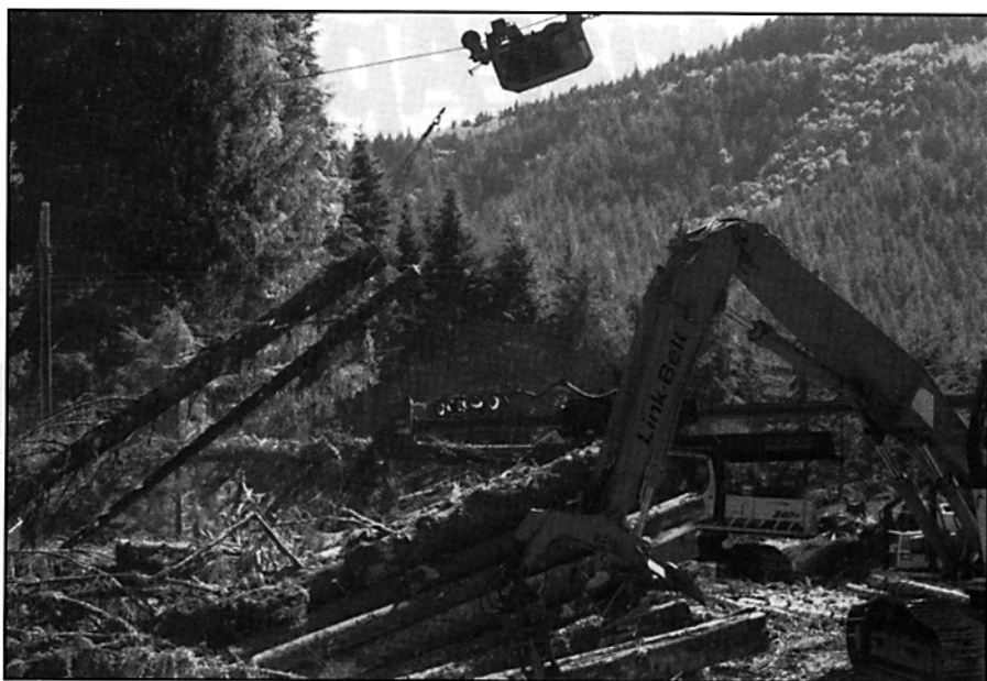
A LANDING IS AN ACTIVE PLACE; ON THE F & B LOGGING TOWER SIDE, LOGS COME IN BY CABLE, ARE DELIMBED AND CUT TO LENGTH, THEN MERCHANDISED AND LOADED. BECAUSE EVERYTHING MUST BE ORCHESTRATED FOR MAXIMUM EFFICIENCY, THE EQUIPMENT CHOSEN MUST BE RELIABLE, FAST, AND EFFECTIVE.
