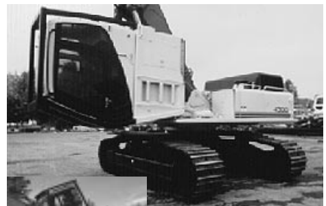
Cab completely tilts forward for ease of transportation and servicing. Hydraulically controlled from side of upper.
